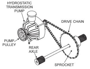
Figure 8. Hydrostatic Transmission
